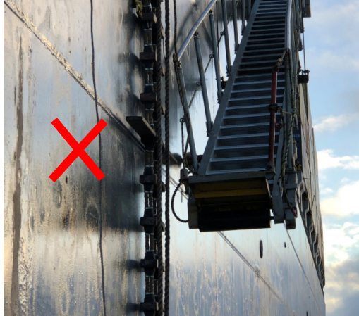
Accommodation Ladder to be secured to ship's side.
